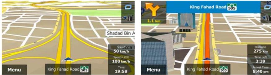
The data fields are different when you are navigating an active route and when you have no specified destination (the orange line is not displayed).
